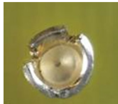
Figure 4: Example of a poorly-formed swage
